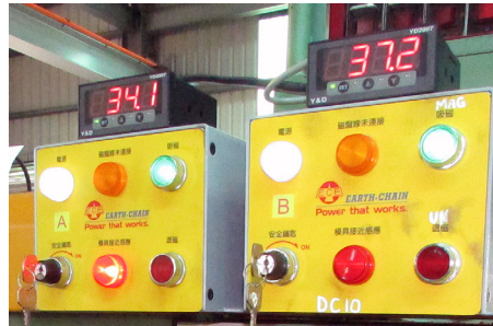
Controls require operator to use both hands.
