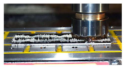
Our 35MM pole chucks are built specifically for the machining of thin workpieces. They are a great choice for drilling, milling, and boring operations on either vertical or horizontal mills. They easily integrate with pallet changing and tombstone systems.
