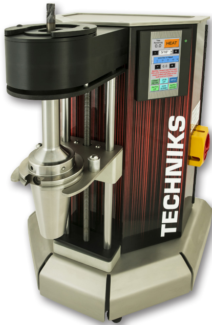
Model 00450 ShrinkSTATION width 16" x depth 16" x height 22" - Weight: 60 lbs
