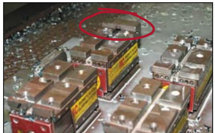
Workstops are used for fast and easy part alignment. (circled) The soft jaws of the magnets have been machined to create clearance for drilling and tapping operations.
