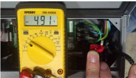
Voltage test of incoming power supply.
