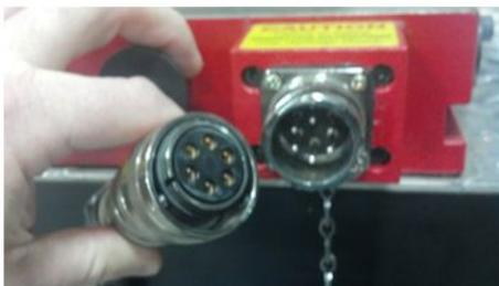
Clean chuck cable and chuck connectors.
