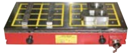
part nests machined into a subplate provide workstops for repeat jobs.
