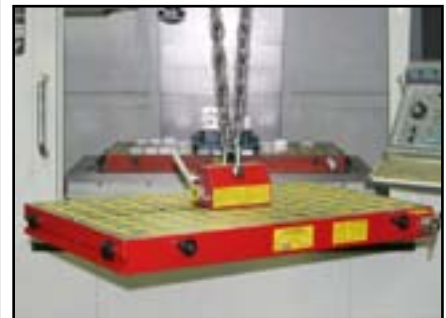
transporting the EEPM chuck
