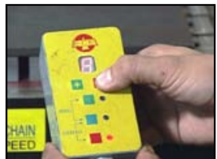
use the + and - buttons to increase or decrease the magnetic power setting
