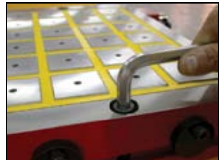
securing EEPM chuck to bed "T" slots
