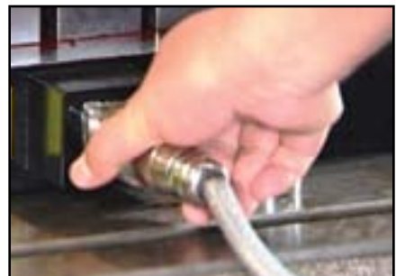
chuck electrical receptacle
