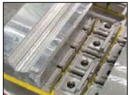
Use induction blocks as work stops
