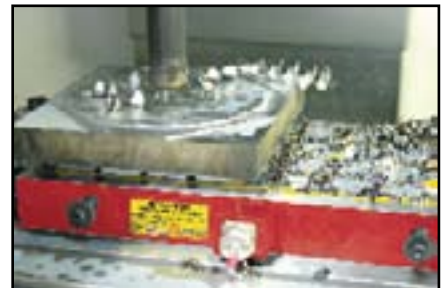
thru-hole application using fixed induction blocks
