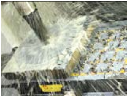
Flood coolant hole making application
