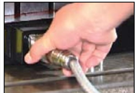
chuck electrical receptacle
