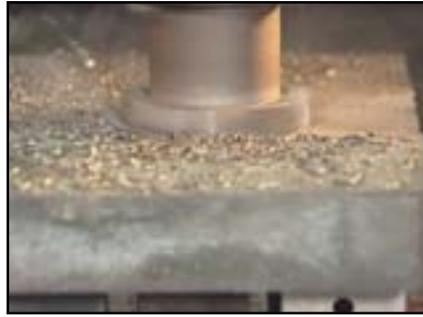
Face milling warped stock
