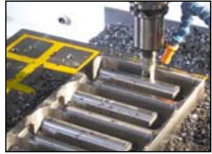
Works great for machining mold cavities
