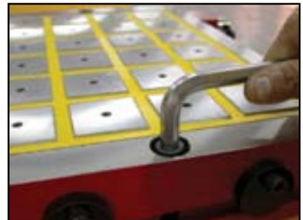
securing EEPM chuck to bed "T" slots
