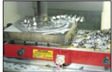
thru-hole application using fixed induction blocks
